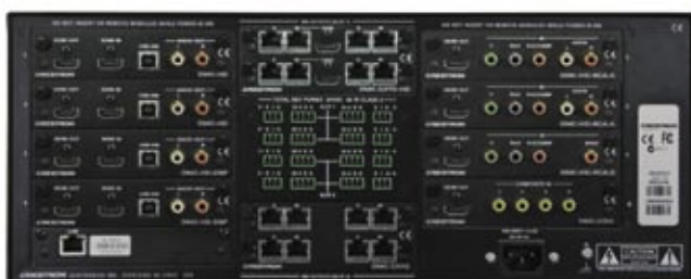
Crestron has got switching taped (8x8 switcher shown). Transmission of HDMI might seem like a black art but the combination of Crestron DM switchers and Digital Media cabling offers two-way data flow complying with HDMI, USB and control information, plus instant source switching too
